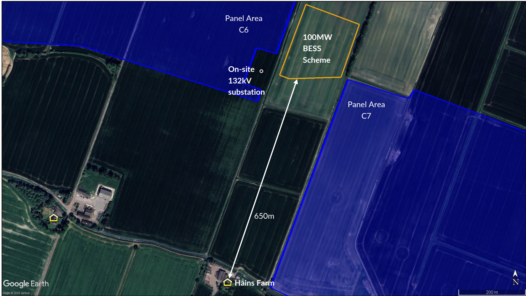
Figure 7 Minimum distance between BESS and the nearest dwelling
